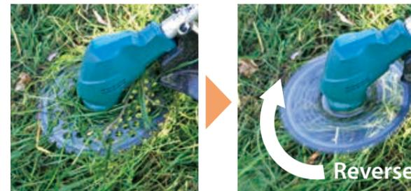
Equipped with reverse switch for easy removal of grass clippings stuck on the blade; grass clippings can be removed from and around the blade by slow reverse rotation of the blade.
