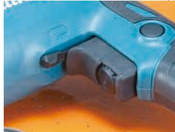
Trigger switch with variable speed control function by dial
