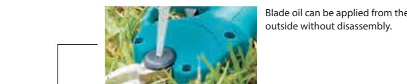
Blade oil can be applied from the outside without disassembly.
