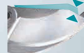
Cutting depth can be adjusted after blade replacement.
