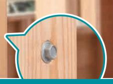
Delivers excellent fastening performance in heavy-duty tasks, such as tightening hex head or hexalobular (star-shaped) hole head course thread screws, which are less prone to cam-out.
