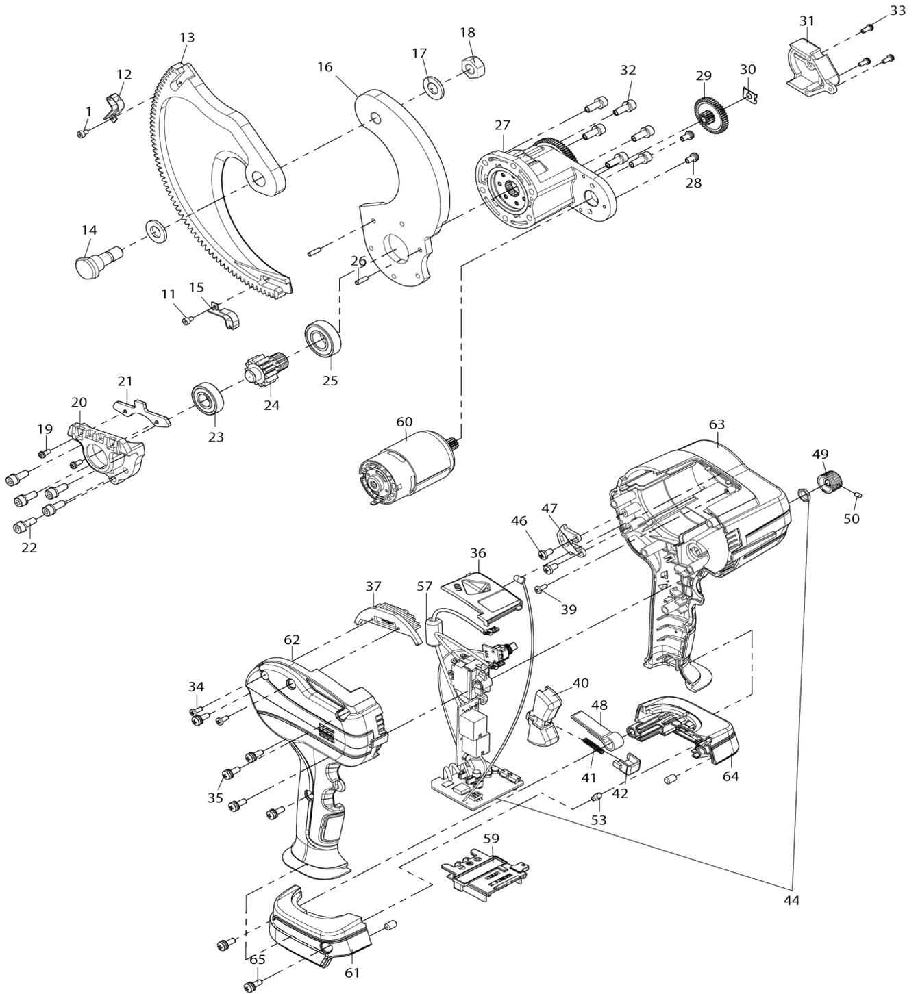
Model No.DTC102 CORDLESS CABLE CUTTER
