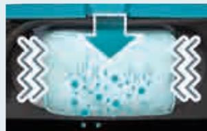
The filter vibrates to remove dust adhering to the filter, reducing clogging.
