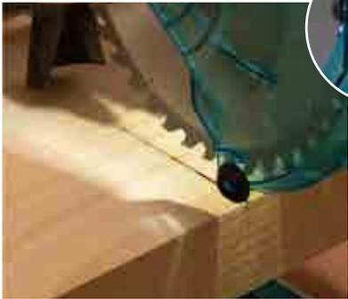
LED job light casts a shadow of the saw blade onto the workpiece as an exact cutting line. By aligning the shadow with the ink line on the workpiece, you can make an exact cut.
