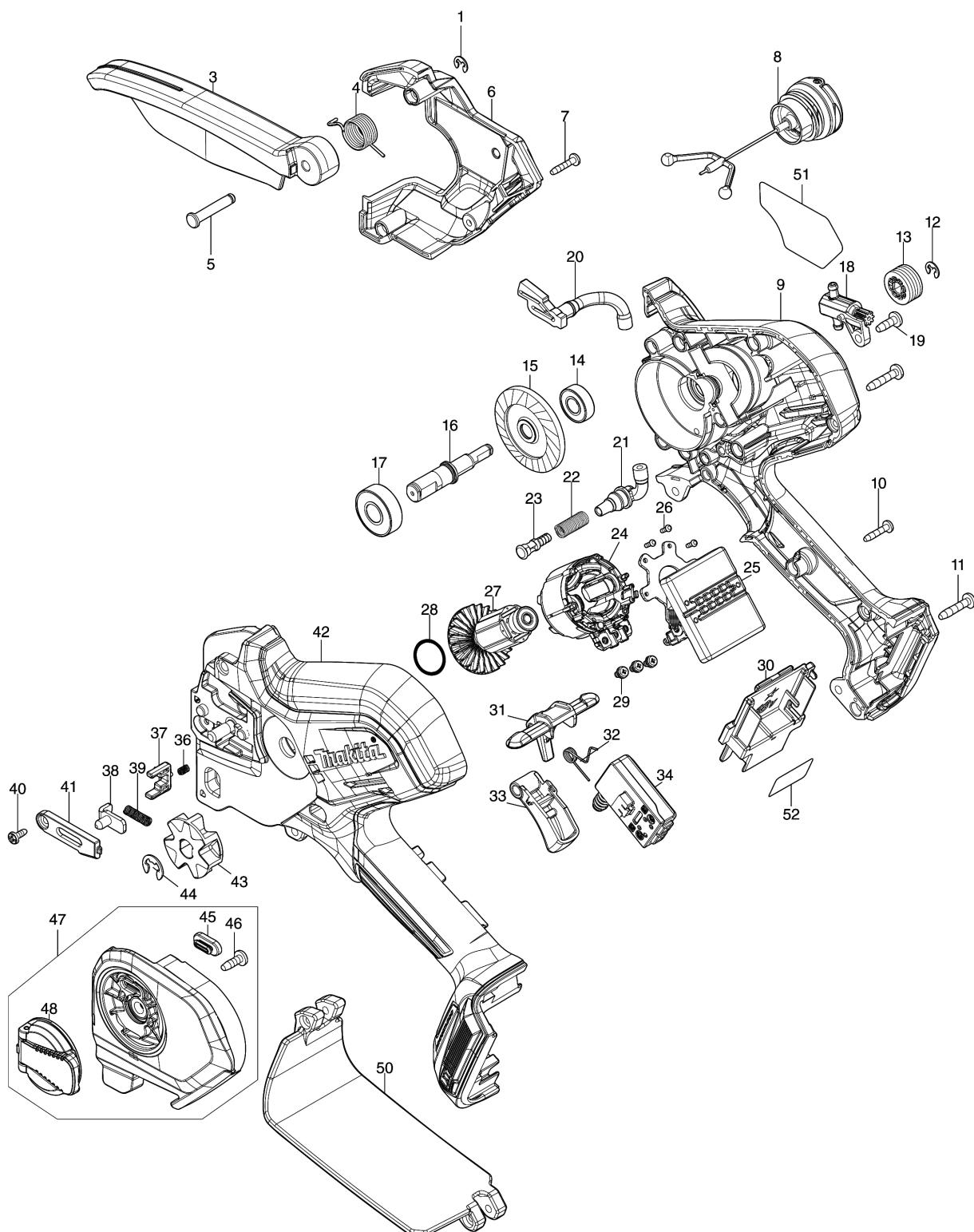
**Model No.DUC101 100MM CORDLESS CHAIN SAW**
