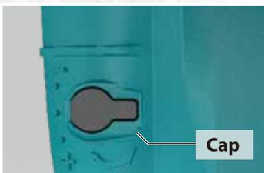
Adjustable automatic chain lubrication
