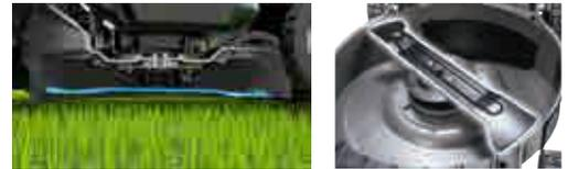
The blade is designed so that it tilts towards the front side of the mower when attached, preventing double-cutting for reduced current consumption.
