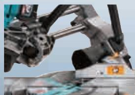
LED lamp casts a shadow of the saw blade onto the workpiece as an exact cutting line. By aligning the shadow with the ink line on the workpiece, you can make an exact cut.
