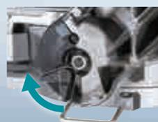
Pull the carriage back slightly and turn the releasing lever for 48° bevel angle in clockwise direction.
