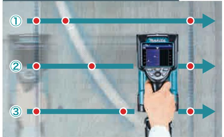
Hold the scanner against the wall surface.
