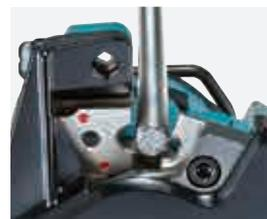
**Automatic blade stop mechanism**
